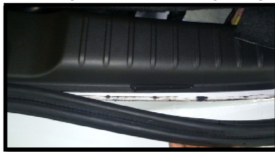
Fig.6. Improper fitment of weather strip
