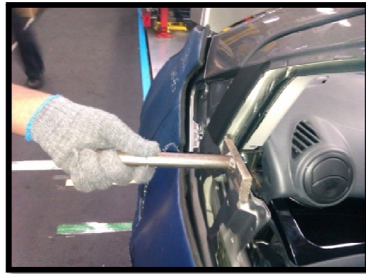
Fig. 9. Implementation of inspection gauge for door water leakage
