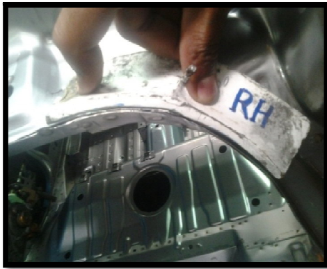
Fig. 8. Implementation of inspection gauge for tailgate water leakage
