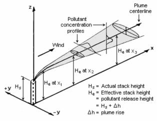
Visualization of a buoyant Gaussian air pollution dispersion plume as used in many atmospheric dispersion models
