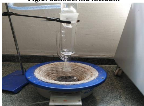
Fig. 2: Ganoderma solvent Extraction using Soxhlation method
