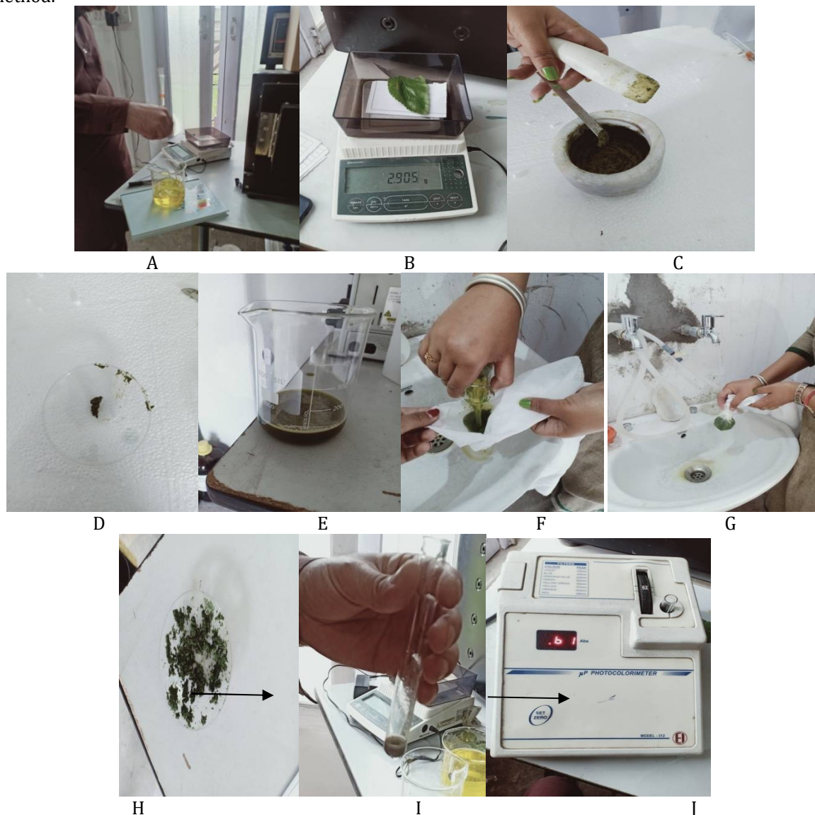
Fig-02: A-J (a:preparation of reagents, b: weighing of leaf tissue, c: grinding of leaf sample, d: Poeredere leaf tissue, e: adding the leaf sample into reagent solution, f: sieving through musslen cloth, g: washing under tap water, h: air dringy the sample, i: tranfering to the burret soultion anf j: sample analysis on photocalori meter) Steps carried out during protein estimation by Biuret Method.
