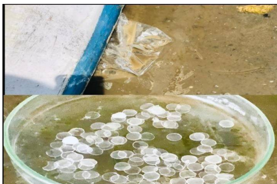
Figure 1: Plastic bag was cut into microplastics with diameter less than >5mm.
