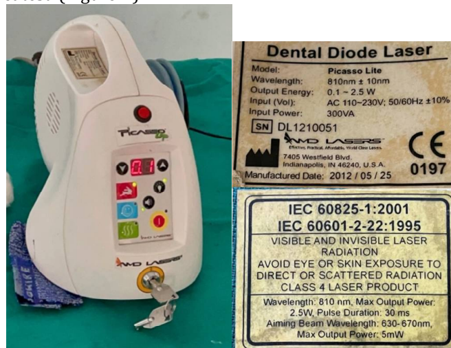
FIGURE-1: DIODE LASER (810nm, Power output:0.1W-2.5W)
