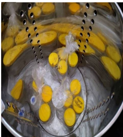
Figure 4 Sterilization of media in autoclave at 121 o C and 15psi for 15 to 20 minutes
